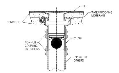
Z1099 shown installed on the outlet of a floor drain. In order for the Z1099 to operate properly, it must always be installed in a vertical position as illustrated.
